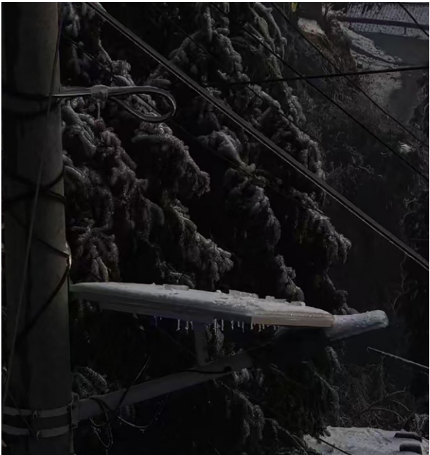
Single-side charging solar energy because the product is covered by snow and ice for a long time, it cannot be charged, cause product damage.
